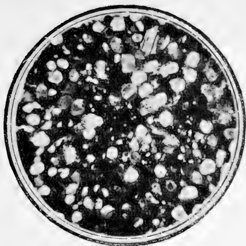
Fig. 8. Lithiumorthosilicate. (Enlargem. 50 times; in immersion-liquid).
